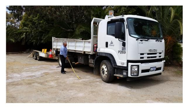
Option 3: was to upgrade to a 9 tonne Isuzu tipper and that would give us a maximum towing weight of 9 tonne. I travelled to Albany City Council to look at their unit. It was a good set up but the truck being on 22inch wheels and the sub frame under the tipper makes it too high for the maintenance crew to work out of the back, remembering we have had two claims and payouts in the last three years with shoulder injuries.
