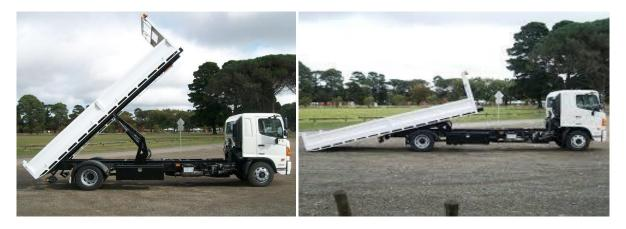
Tiltip was option 6: This unit is very versatile. It has multiple uses especially in local government. Still low enough to work out of in the smaller classes of trucks. Still a bit limited in the weight it can carry. If it were to replace the existing 6 tonne truck with a FVD1000 it can do the job on the
