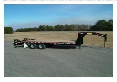
Option 4: I looked at a gooseneck configuration. This would help load share to the truck, so I thought. Transport Department were very unclear on the configuration but at first they thought it could work. On second attempt to get more clarification they still felt it broke the rule of towing 5 tonnes even though it load shared.
