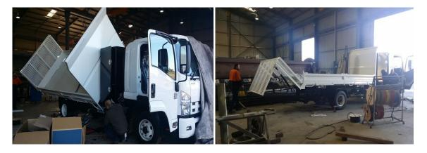
Remembering the first option was for the maintenance truck to be a side tipper with hydraulic ramp at the rear.
